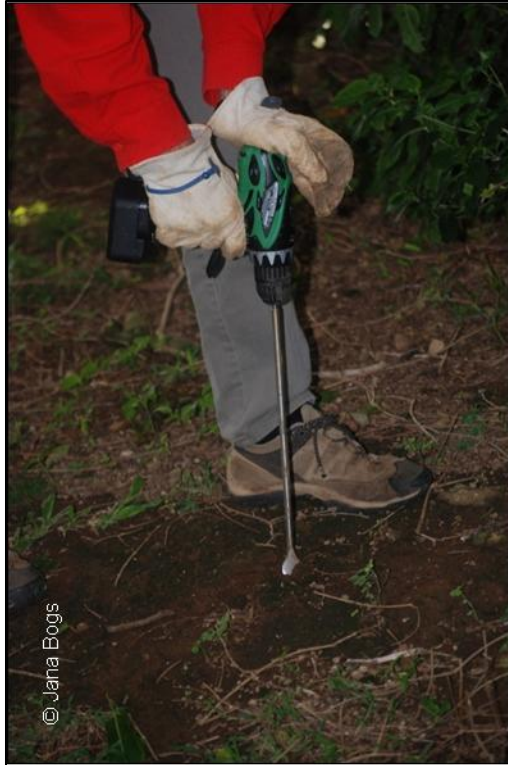
Battery-powered drill with long, wide-tip drill bit for difficult soils
